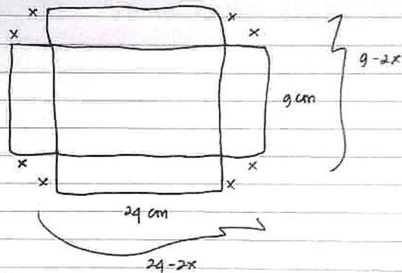
$$\begin{aligned} V &= p \times l \times t \\ &= (24 - 2x)(9 - 2x)(x) \\ &= 4x^3 - 66x^2 + 216x \end{aligned}$$
